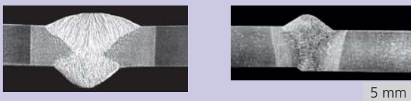
Polished cross section and strength values of a MSG/UP weld seam compared to a laser hybrid weld (SZW Union NiMoCr).
